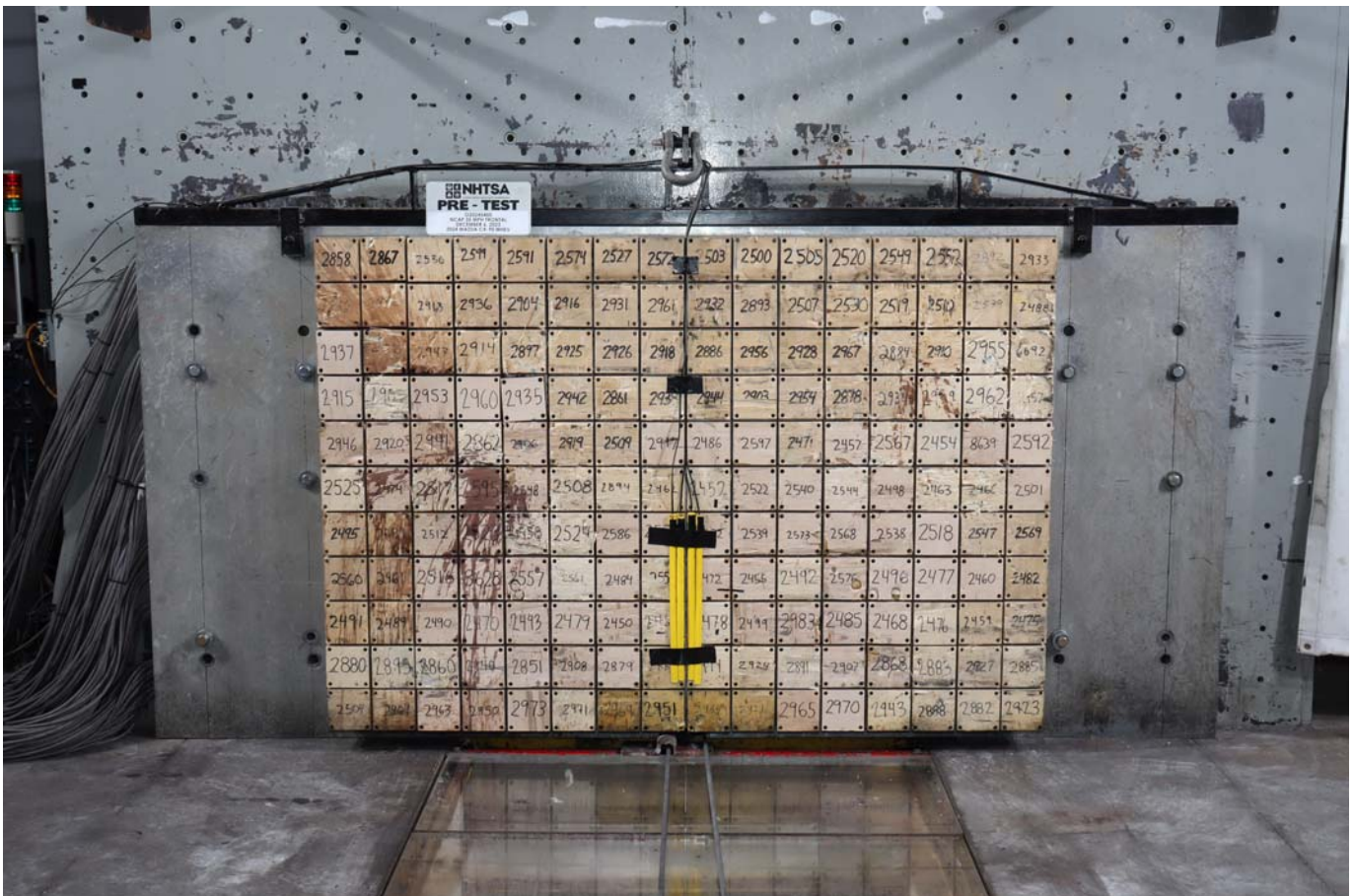
Photo No. 002 - Pre-Test Load Cell Wall
